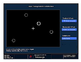
For a case where multiple relationships would display, consider an input of 1080p/23.98 Hz with a reference of NTSC/59.94 Hz:
