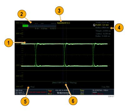
At the end of a long cable, the eye diagram may appear so noisy that there is little or no discernible opening. In this situation, limited use of the eye diagram is still possible by selecting Equalized Eye mode. The equalizer compensates for the effects of cable length by applying an inverse response function and then reslicing the signal to a logic level. This causes amplitude information to be lost, but preserves the effects of jitter in the signal.
