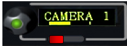
Figure 5-4: Rotary panel display: latched listen while talking
