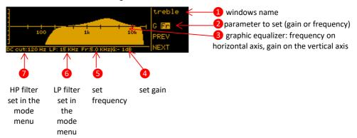
For each window it is showed the graphic equalizer which help to see the set parameters. Push the rotatory knob to change the parameter between gain and frequency (the respective letter G or Fr is highlighted during the setting phase) and
