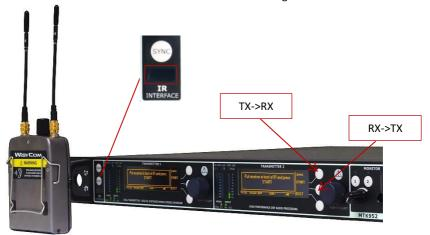
Press the SYNC button on the transmitter: the following message is showed on both the displays
