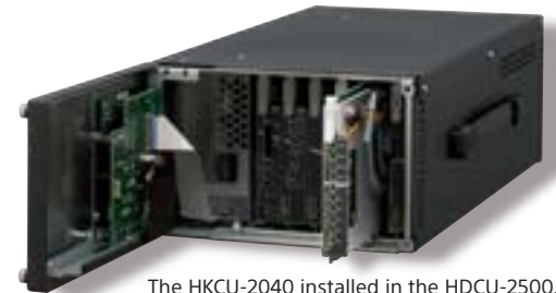
The HKCU-2040 installed in the HDCU-2500.
