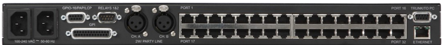
Figure 2. Rear of the Zeus III has two-wire partyline connectors
